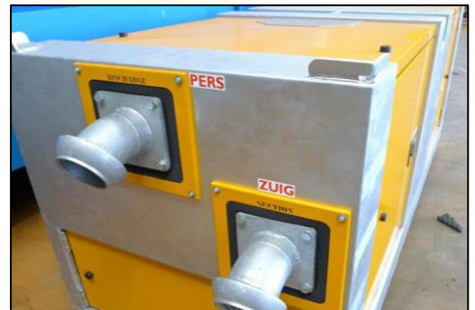
The panels are 2 cm inside in the frame to prevent damaging during transport.
