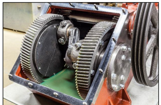
The single, high-precision gears ensure quiet operation.
